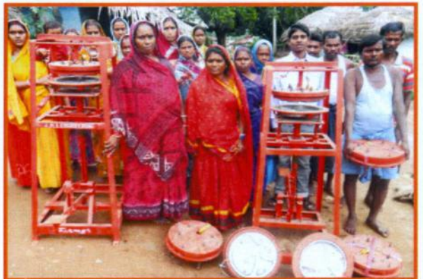
Improved four sections plate die
